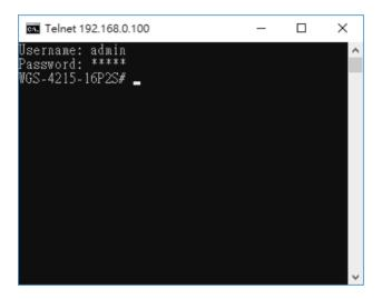
Figure 6-1: Wall-mount Managed Switch Telnet Login Screen
